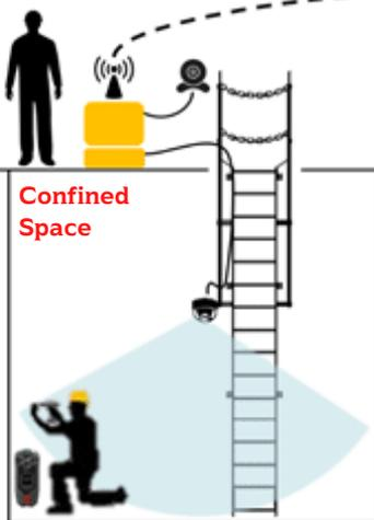
**3** Worker carrying a 4-in-1 gas detector, the reading and alarm will be sent to the cloud platform in real-time basis, and also will be shown on the monitoring station
